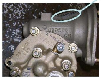
FIGURE 1. Example of Vibro-Peened Manufacturer Code
