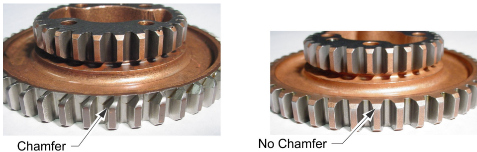
Figure 4. Chamfer Tooth Gear Profile
